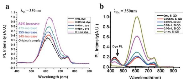
**Fig. 4** (a) The PL trend of a certain amount of SiQDs with different amounts of VA co-encapsulated in micelles. (b) The change of PL of a certain amount of VA with a different amount of SiQDs co-encapsulated in micelles.
