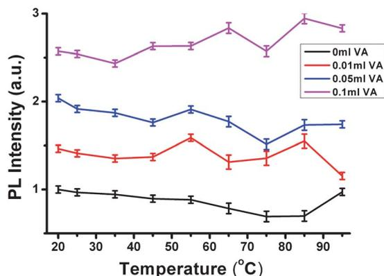
**Fig. 7** PL of MSiQDs-VA under different temperature.
