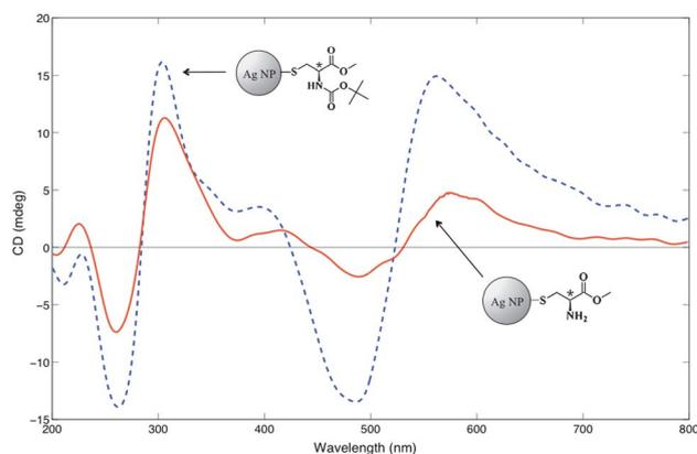
**Fig. 4** Representative CD spectra of *t*-BOC protected Ag NP film (blue line), and *t*-BOC deprotected Ag NP film (red line).
