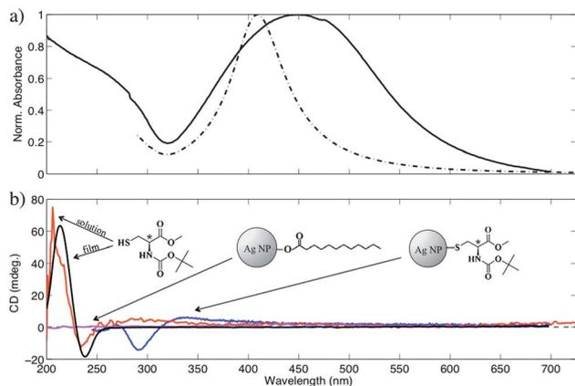
**Fig. 2** (a) Absorption spectra of *t*-BOC Ag NP film (solid line) and dispersion in chloroform (dotted line); (b) CD spectra of *N*-(*tert*-butoxycarbonyl)-*L*-cysteine methyl ester dissolved in ethanol (red line), and as a film (black line), dodecanoic acid protected Ag NPs (as a film, magenta line), and *t*-BOC protected Ag NPs dispersed in chloroform (blue line).
