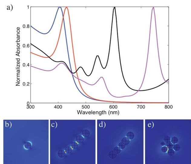
**Fig. 3** (a) Normalized absorbance spectra of an isolated silver nanoparticle (10 nm size) and different configurations of Ag NPs clusters: single Ag NP (blue line), chain of 5 Ag NPs (red line), cluster of 5 Ag NPs (black line), and cluster of 9 Ag NPs (magenta line); (b)–(e) cross-sectional plots of the norm of the electric field at  $z = 0$ . In each case (b through e) the wavelength corresponds to the maximum value of absorbance.
