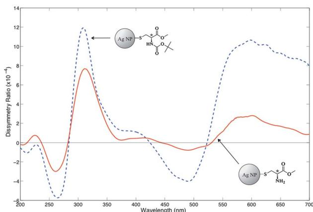
**Fig. 5** Absorbance dissymmetry ratio of *t*-BOC protected Ag NP film (blue line), and *t*-BOC deprotected Ag NP film (red line).
