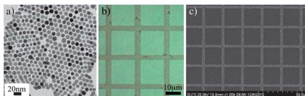
**Fig. 1** (a) TEM image of Ag NPs, (b) optical and (c) SEM image of two-photon patterned Ag NP films.
