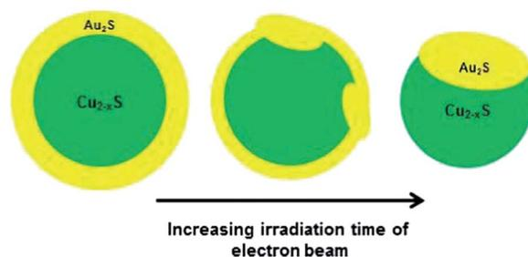
Fig. 8 Schematic illustration of the apparent mechanism of morphological transformation of a  $\text{Cu}_{2-x}\text{S}-\text{Au}_2\text{S}$  core/shell NC to a  $\text{Au}_2\text{S}$ -tipped  $\text{Cu}_{2-x}\text{S}$  NC by electron irradiation.
