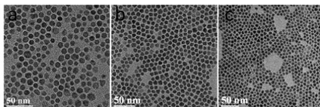
Fig. 1 TEM images of (a)  $\text{Cu}_{2-x}\text{S}$  NCs used as templates, (b)  $\text{Cu}_{2-x}\text{S-Au}_2\text{S}$  NCs produced by cation exchange using 0.056 mmol Au precursor (nominal 1 : 4 Au : Cu ratio), and (c)  $\text{Au}_2\text{S}$  NCs produced by cation exchange using 0.3 mmol Au precursor (nominal 4 : 3 Au : Cu ratio).
