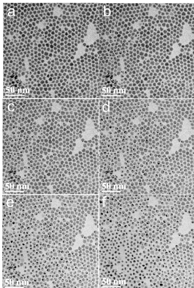
Fig. 6 Still images from a TEM recording of the morphological transformation of  $\text{Cu}_{2-x}\text{S}-\text{Au}_2\text{S}$  core/shell NCs upon electron beam irradiation. (a) Initial configuration of  $\text{Cu}_{2-x}\text{S}-\text{Au}_2\text{S}$  core/shell structure. (b)–(f)  $\text{Cu}_{2-x}\text{S}@-\text{Au}_2\text{S}$  to  $\text{Au}_2\text{S}$ -tipped  $\text{Cu}_{2-x}\text{S}$  nanoparticles. Images were recorded at 15 s time intervals over a period of 90 s.
