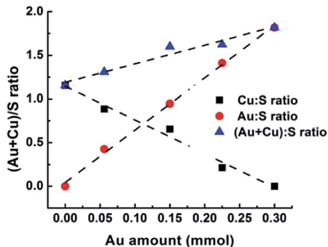
Fig. 3 Dependence of copper, gold, and total cation content (relative to sulphur content) on the amount of Au precursor provided.
