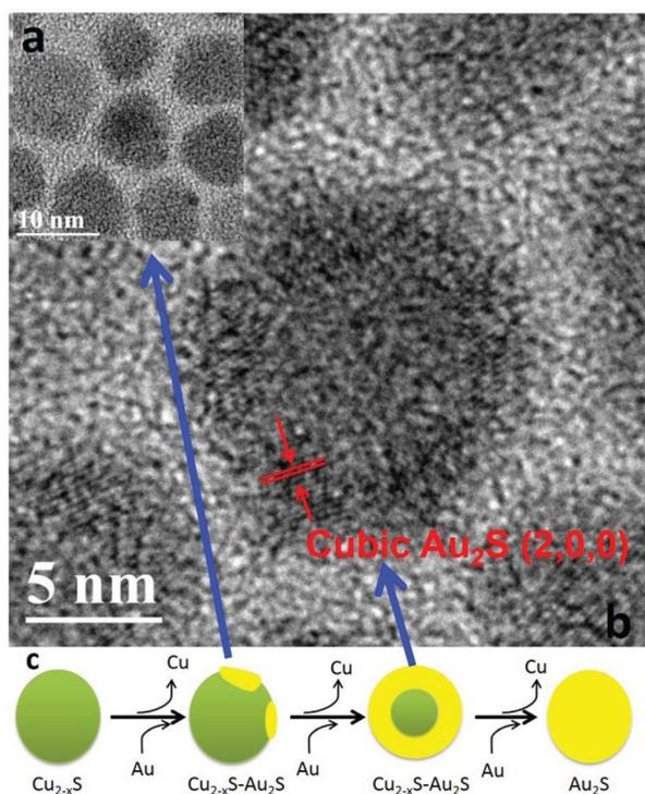
Fig. 2 HRTEM images of NCs obtained after (a) cation exchange using 0.056 mmol Au precursor (nominal 1 : 4 Au : Cu ratio), and (b) cation exchange using 0.225 mmol Au precursor (nominal 1 : 1 Au : Cu ratio); (c) schematic illustration of the cation exchange process.
