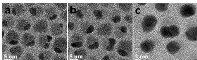
Fig. 7 HRTEM images of  $\text{Cu}_{2-x}\text{S}-\text{Au}_2\text{S}$  structural transformation under electron beam irradiation.
