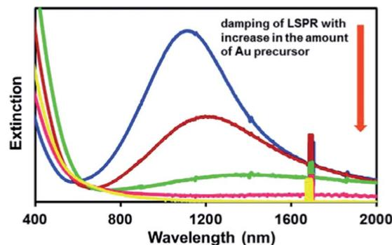
Fig. 5 Optical extinction spectra illustrating LSPR of template  $\text{Cu}_{2-x}\text{S}$  NCs (blue) and cation-exchanged NCs following reaction using 0.056 (red), 0.150 (green), 0.225 (pink) and 0.300 (yellow) mmol Au precursor corresponding to Au : Cu ratios of 1 : 4, 2 : 3, 1 : 1, and 4 : 3, respectively.
