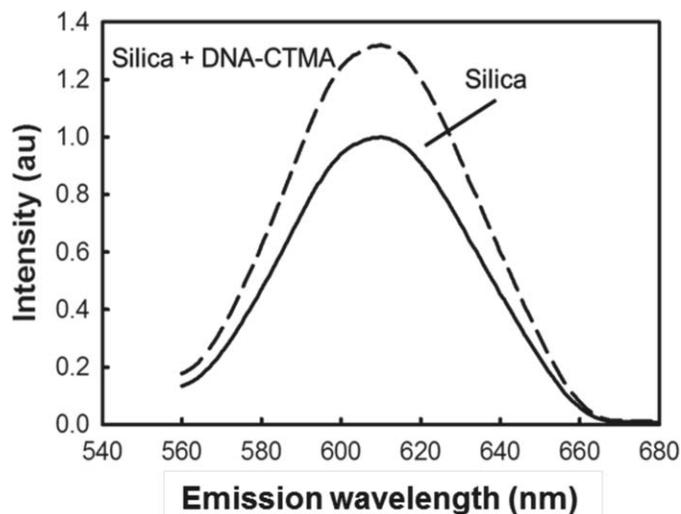
FIG. 3. Luminescence emission spectra for  $[\text{Ru}(\text{dpp})_3]^{2+}$  sequestered within silica-only and silica-DNA-CTMA xerogels.
