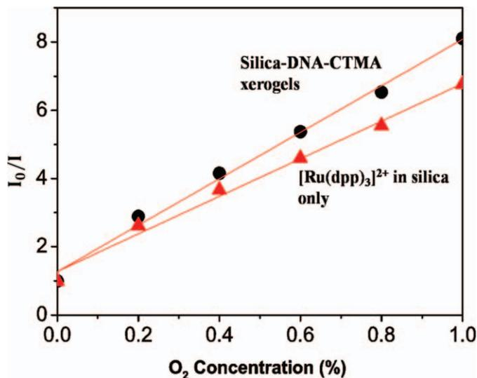
FIG. 4.  $\text{O}_2$  Stern–Volmer plots for  $[\text{Ru}(\text{dpp})_3]^{2+}$  in silica-only and silica-DNA-CTMA xerogels.
