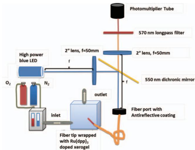
Fig. 2. Hybrid quenchemetric DNA-silica xerogel sensing platform measurement setup. The xerogel sensor is coated on the fiber in the measurement chamber and the light emitted from the xerogel is carried by the fiber to the PMT.
