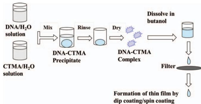
Fig. 1. Process procedures of DNA-CTMA complex.
