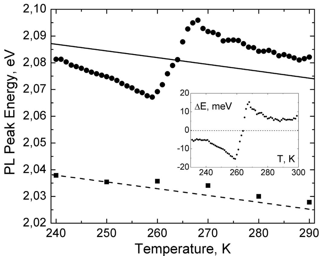
**Figure 3** PL peak energy of (squares) dry colloidal CdSe NPs sample and (circles) in-liquid CdSe/ZnS NPs. The insert shows the same dependence for in-liquid NPs without monotonic part introduced in Equation 1.
