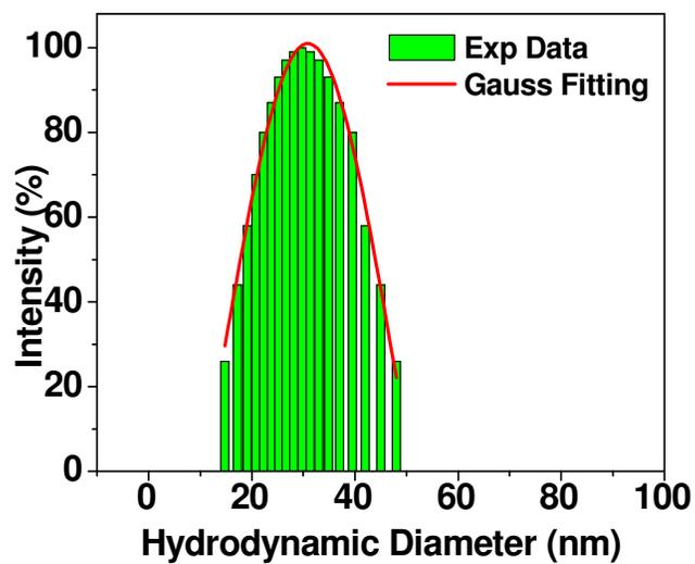
**Figure S2.** Hydrodynamic diameter of ligand-free (NaGdF<sub>4</sub>:3% Nd<sup>3+</sup>)/NaGdF<sub>4</sub> core/shell nanocrystals.
